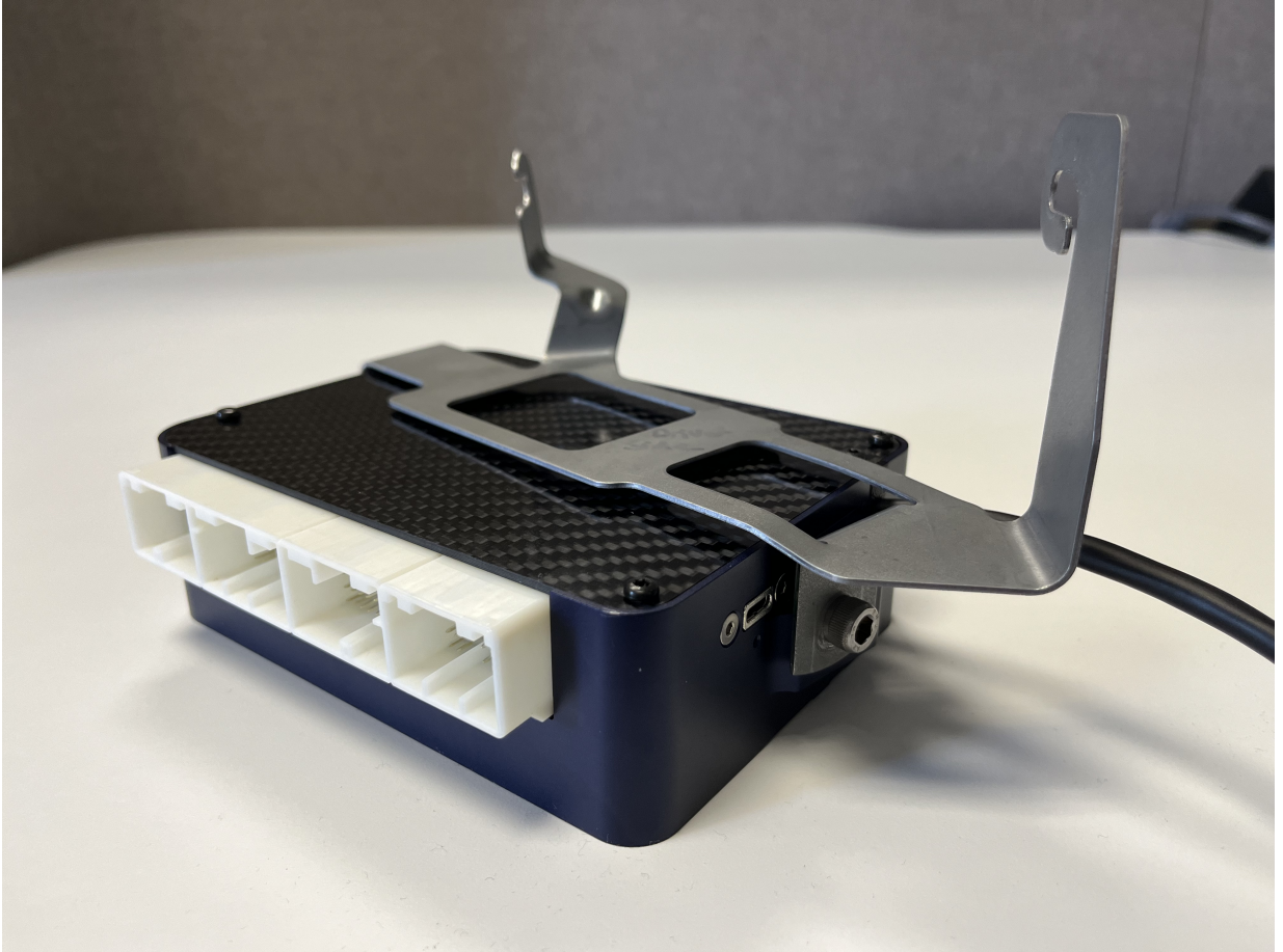
Link PNP ECU on OE bracket
